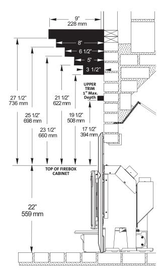
Figure 6. Minimum Mantel Clearances. Measure clearances from the top and sides of the fireplace cabinet before installation of the cast iron surround panels.
